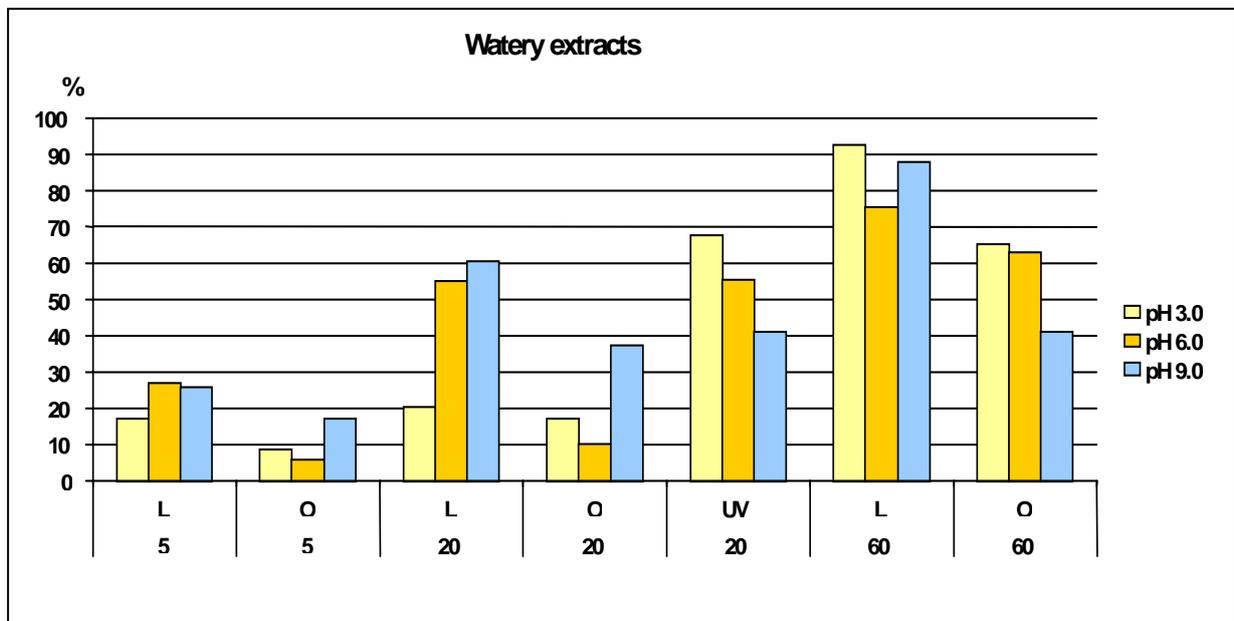
**Figure 3.** Color losses of watery and ethanolic extracts after 21 days of storage, expressed like % absolute absorbance losses at 430 nm. L -solar light, O-darkness, UV- UV light, the practiced temperatures 5°C, 20°C and 60°C
